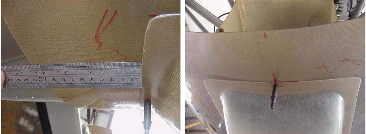
Use 3" screw spacing on the scoop with a screw in each corner. Rear screws are the same as duct mount screws. Screen is installed after painting with 8 8-32 screws and nuts. A vertical brace from top to bottom of the screen at the center is a good idea for strength.
